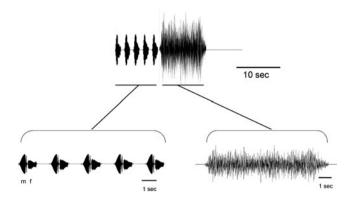
**Fig. 3** Example stimulus used to test male responses to wind. A duet consisting of four alternating male and female signals was used to elicit male signaling. Plant vibrations were induced using a fan
